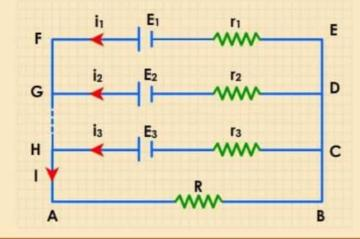
$$I = \frac{\sum\limits_{\substack{i=0\\1+R}}^{n}\frac{E_{i}}{r_{i}}}{1+R\sum\limits_{\substack{i=1\\i}}^{n}\frac{1}{r_{i}}} \text{ and } E_{eq.} = \frac{\sum\limits_{\substack{i=1\\r_{i}}}^{n}\frac{E_{i}}{r_{i}}}{\sum\limits_{\substack{i=1\\r_{i}}}^{n}\frac{1}{r_{i}}}, \quad r_{eq.} = \frac{1}{\sum\limits_{\substack{i=1\\r_{i}}}^{n}\frac{1}{r_{i}}}$$
